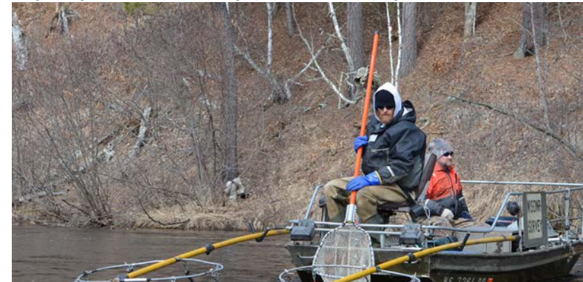
Below: Mini-boom electrofishing on a river in northern Wisconsin. This type of sampling is designed to get into shallow water and tight places, like when sampling the Yahara River.
