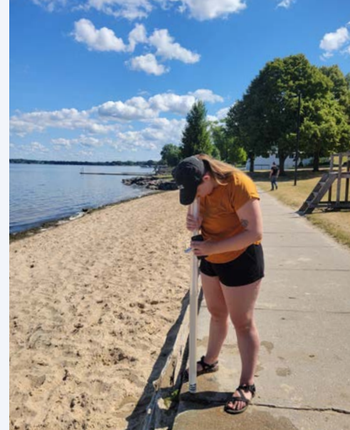
Clean Lakes Alliance volunteer water quality monitor uses a turbidity tube to measure near-shore water clarity, 2023
