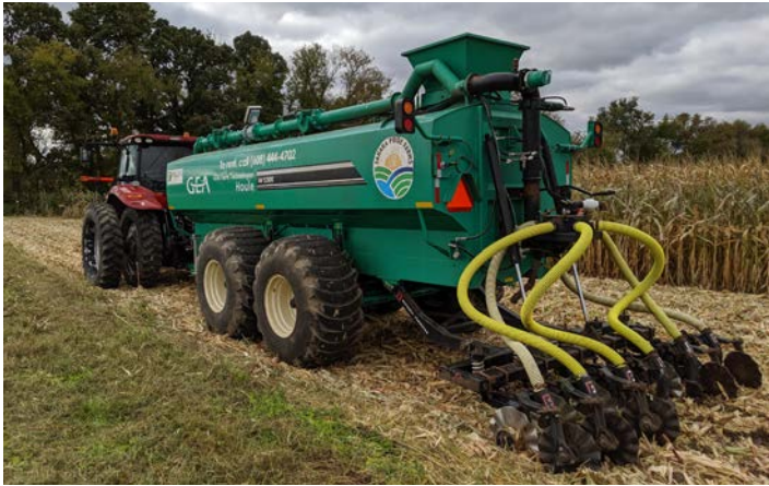
Photo: Low-disturbance manure injection is an example of a conservation practice farmers use to help prevent manure from washing off fields.
